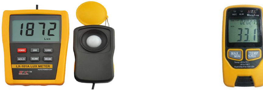
Figure 10 HTC Lux Meter: LX101A/LX102A (left) and Easy Log -RH- Temp data logger (right) (Source: Author)
