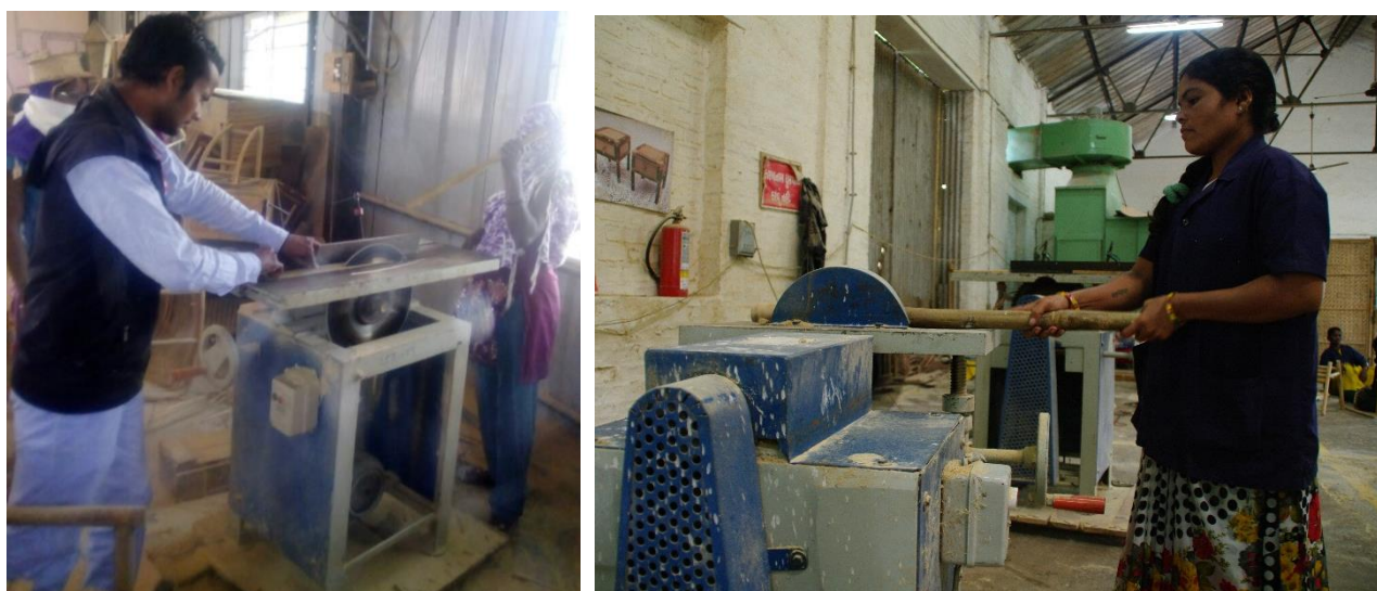
Skilled Manpower: Removing Knots in Bamboo Pole
